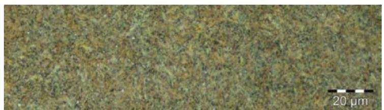
The microstructure of the induction hardened layer is low tempered martensite and small carbides (magnification 500x) – 5 Cr steel.
