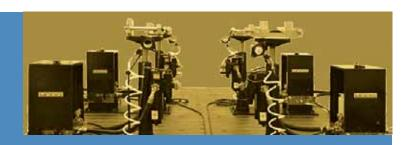
The system incorporates fatigue-rated hydrostatic servo hydraulic actuators for specified vertical accelerations up to 45 g.
