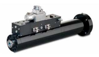
The Moog model LH11RS series or the Moog Hydraulic Actuators with hydrostatic bearings are employed in the Tire Coupled Simulation Systems. Hydrostatic bearings allow for higher side loading capability without damage to rod or bearing end cap surfaces. Up to 12 inches of travel accommodate a broader range of vehicle applications from compact vehicles to light duty trucks.
